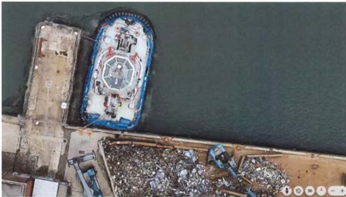
Figure 23: Tug docked at Berth 46 Nib showing blocked access and proximity of cargo operations
