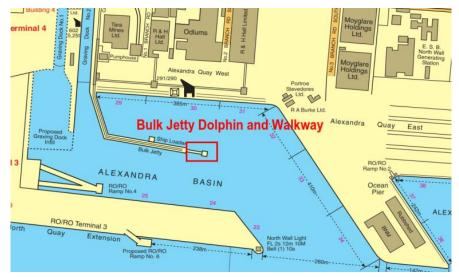
The works generally consist of the demolition of the existing 45m long x 8.0m wide Dolphin and Walkway. The Dolphin Structure consists of a concrete pilecap supported on Tubular Steel Piles.
